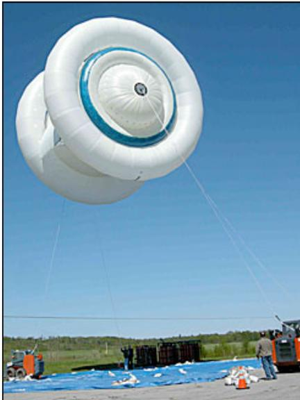
Magenn Power's floating wind turbine is a helium-filled balloon with wings. Wind blowing across it catches the wings, which are its rotors, making it spin, resulting in electricity generation. Tethers hold it in place and transmit the power to the ground. Photo courtesy of Magenn Power.
